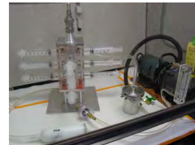
Nose-only inhalation chamber • Expose mice to air pollution or particulate matters
