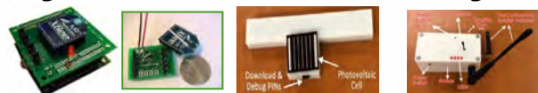
Missouri S&T Mote, RFID tag for networking sensing and decentralized control, diagnostics and prognostics
